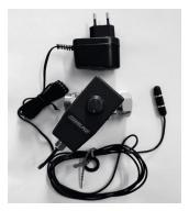
Fig. 78: External water sensor
