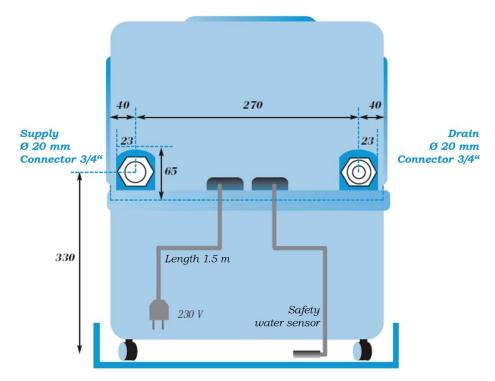
Fig. 58: Automatic flushing device
