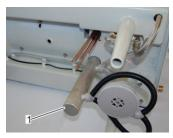
⇒ The UV degermination system is located below the center plate next to the pump (Fig. 66/1).
