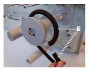
6. Remove the pump hoses (Fig. 38/1).
