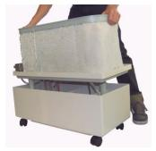
3. Lift the center piece from the water tank and place it to the side (Fig. 44).
