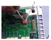
Fig. 21: Coding the humidifier
