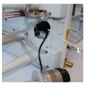
Fig. 48: Disconnecting the plug connection
