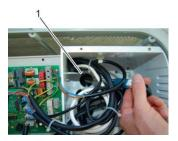
Fig. 74: Pulling out the UV lamp
