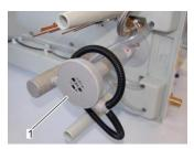
⇒ The water pump is located at the bottom on the righthand side (Fig. 45/1).
