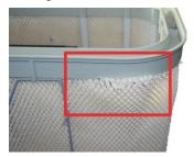
Fig. 30: Incorrect filter placement
