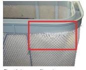
Fig. 10: Incorrect filter placement
